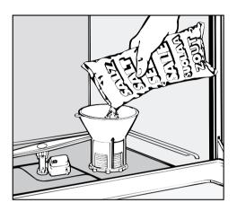
Before adding salt for the first time, fill the reservoir with approximately 1 quart (1 l) of water.
